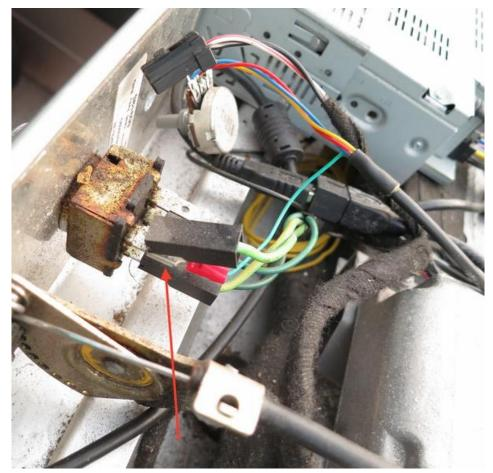
5. Pop bonnet, remove washer fluid tank for better access, unplug cable coming from cabin under heater (or cut if older, hard wired version)
