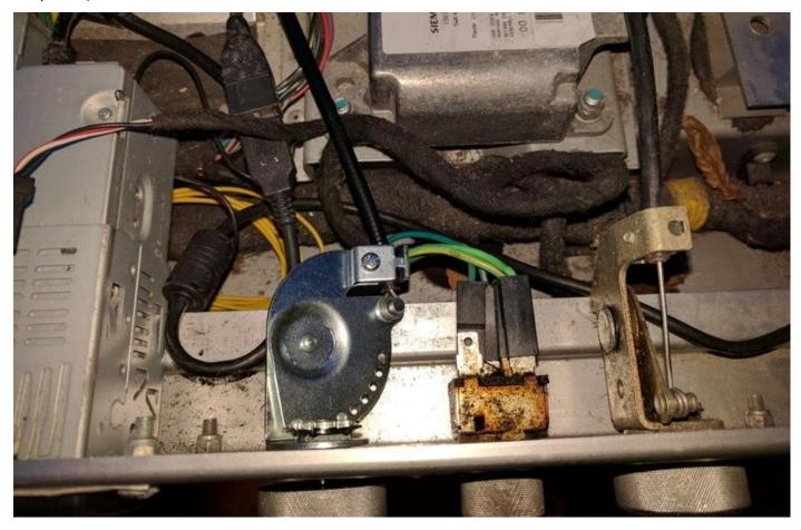
8. At heater end, attach cable end to mechanical valve
